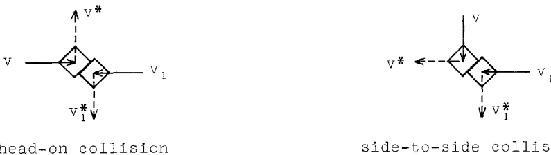
Fig. 1. In our dynamics there are only two (essentially distinct) types of collisions as diagrammed, where v and v_1 ( v^* and v_1^* ) denote the precollisional (postcollisional) velocities.
